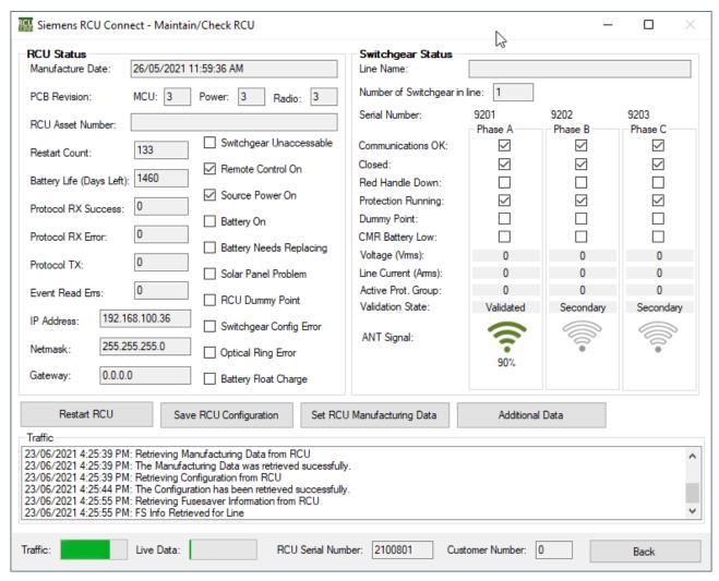
**Fig. 48** *RCU Connect* – RCU communicating correctly with Fusesavers (top) and CMR installations (bottom)
