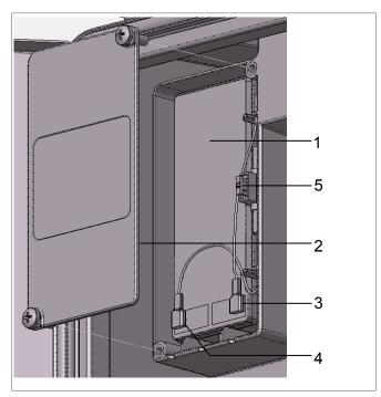
Fig. 17 Battery Connection Details
