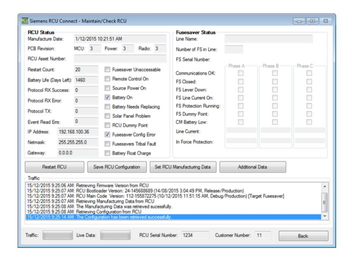
**Fig. 47** *RCU Connect* – Maintain/Check Window for Fusesaver Installations.
