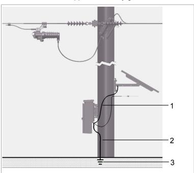
Fig. 30 RCU and Solar Panel Earthing Diagram
