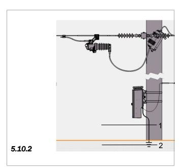
Fig. 29 RCU Earthing Diagram
