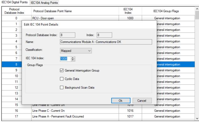
**Fig. 41** *RCU Connect* – Edit Protocol Screen. Top is a DNP3 example. Bottom is an IEC104 example.
