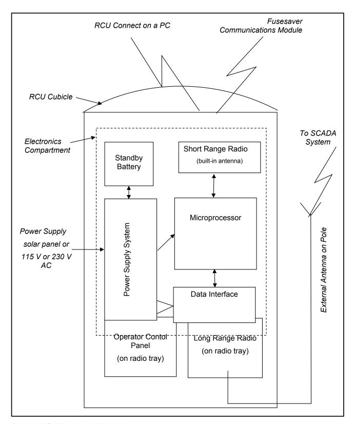
Fig. 12 RCU Functional Block Diagram
