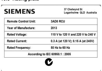
Fig. 53 Example – RCU rating plate
