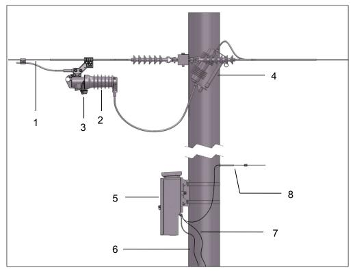
Fig. 2 Installation of RCU with Fusesavers
