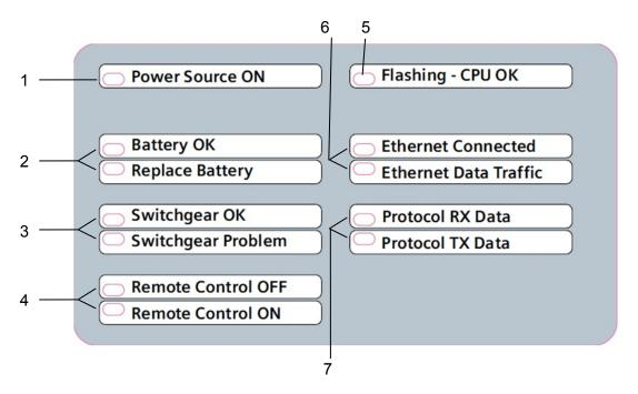
Fig. 6 LED Indicator Display
