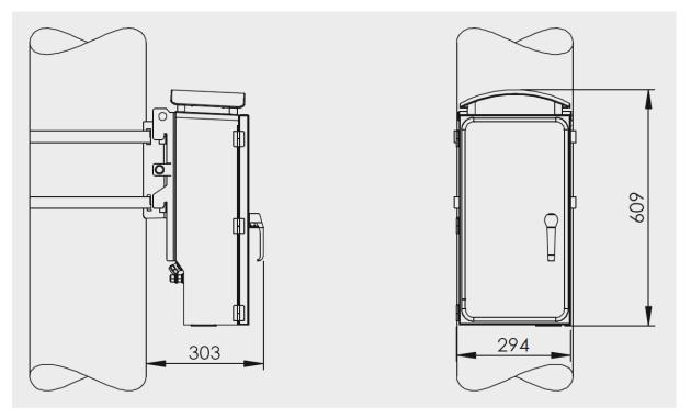
Fig. 54 RCU Dimensions (in mm)
